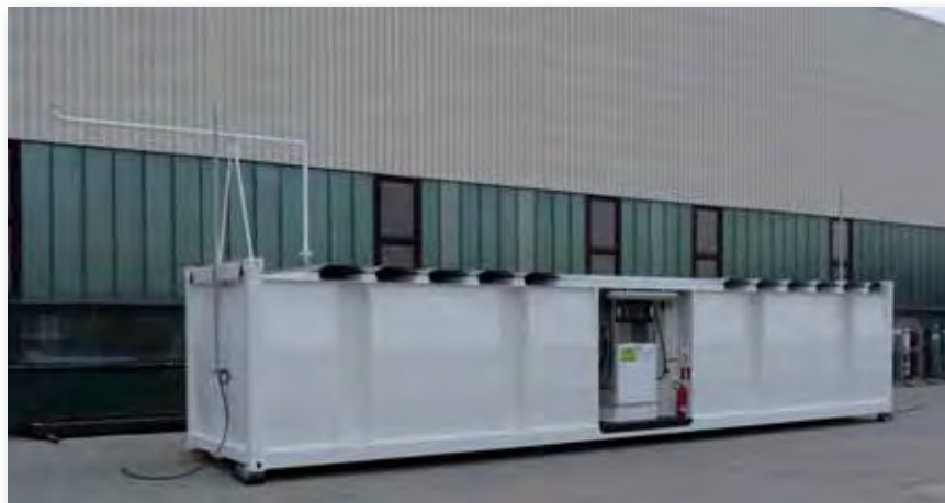
40-foot petrol station container - two-chamber tank with integrated filling pump niche, aggregate niche, lightning protection, ventilation 2 m above tank roof (petrol chamber) and sun roof
